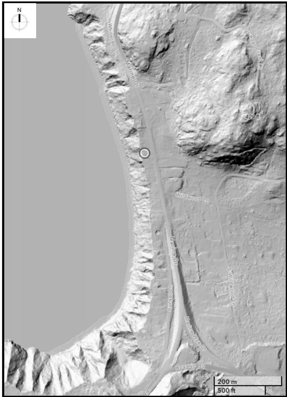
Figure 6: Lidar Imagery 1 showing scalloped ridge crests on the coastal bluff in the vicinity of the project site shown as the black dot. Imagery courtesy of Washington Geologic Information Portal , 2026.
